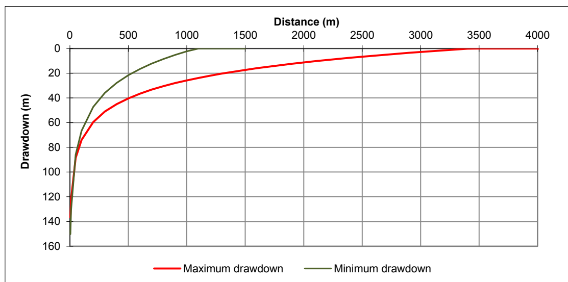
Figure 20-11: Extent of drawdown from the edge of the mine workings after 10 years of mining (Theis, 1935)
