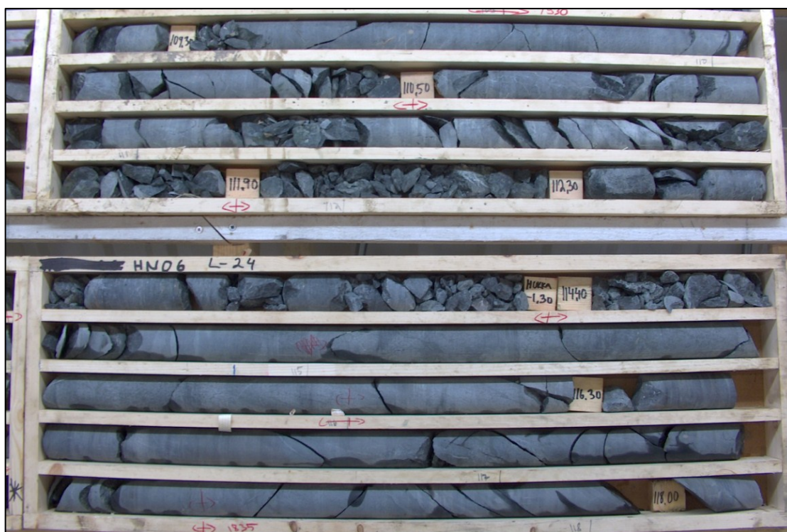
Figure 20-5: HN06 core photo illustrating a zone of intense fracturing
