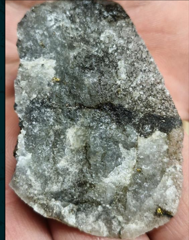
Piece of quartz-chlorite vein with disseminated chalcopyrite and VG (invisible by naked eye); interval returned 1.0m @ 39.7 gpt Au from 408.3m (DH MW09).
